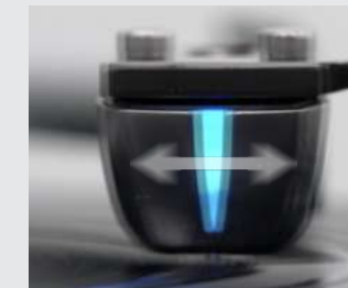
There is eccentricity: Cartridge is forced to sway
